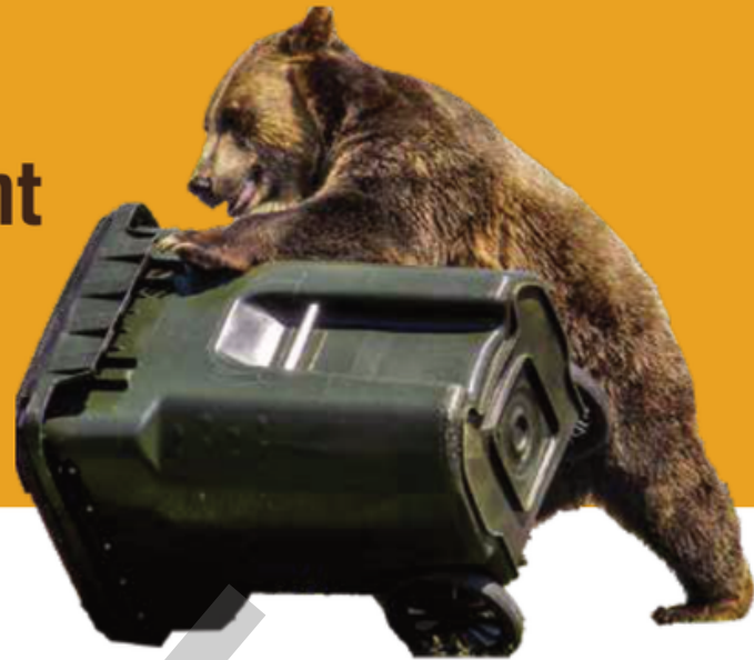
This bear tested a trash can to determine whether it can be certified.
